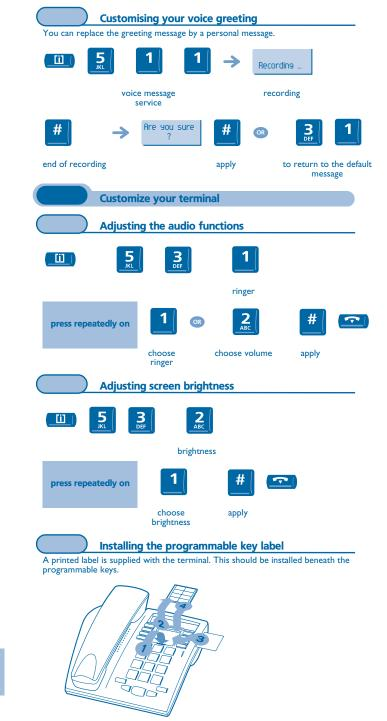
Insert a flat " blade " into the slot (1 slot per key block). 1.
