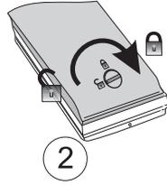
While maintaining the battery module in position, slip the lock to the locked position
