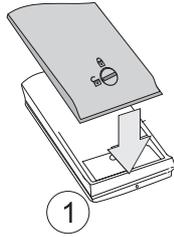
Before inserting the battery module into the phone, make sure that its lock is in the unlocked position
