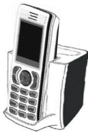
Connect the charger and place the telephone in the charging holder. The battery charger LED lights. The battery LED is in charging mode on the phone screen. If the battery is completely discharged, a charging time of several minutes is required before the set will light up again.
