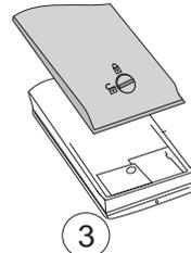
You can then remove the battery module
