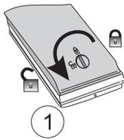
Slip the lock to the unlocked position
