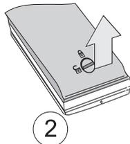
Lift the battery module from the bottom
