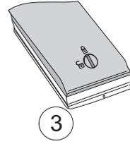
Check that the battery module is properly installed in its housing
