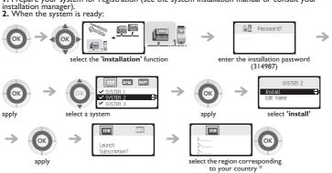
The DECT set can be programmed and can address the 4 specified frequency bands. On installation, the user of a DECT set must declare the set in the appropriate frequency band according to the country in which the user finds himself:
